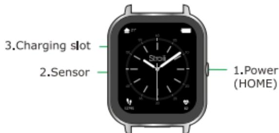
1. Power on/off: long press to power on/off the device; short press to turn on/off the screen.
